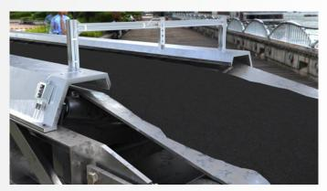
Checking the processing temperature when loading asphalt with thermoMETER UC
