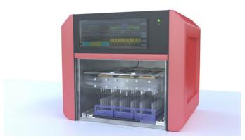
Measuring the temperature of samples in DNA analyzers with thermoMETER FI
