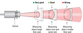
The spot sizes can be changed by selecting the appropriate focus. For example, a CF lens can generate very small spots, while an SF lens generates larger spots, but enables measurements over larger distances.
