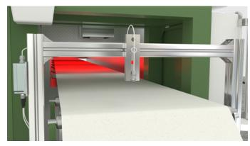
Monitoring the drying process in paper production with thermoMETER UC
