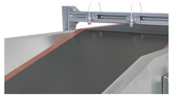
Temperature measurement in the coating process of battery films with thermoMETER UC
