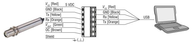
Fig. 6.4: Pin assignment digital output
