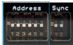
Fig. 63 DIP switch on the MSC7602 for multi-channel operation
