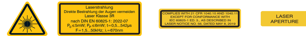
Laser warning sign and laser label, ILD2310-x Only for USA Near laser output
